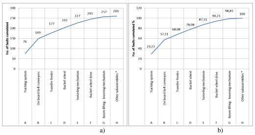
**Fig.2.** Pareto diagram in cumulative frequency of failures expressed in no. of failures, a) and percentage, b)
